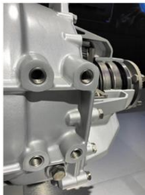
Threaded inserts for motor housing
